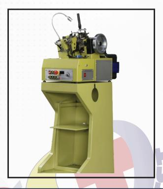
High Speed Chain Making Machine With Laser Welding System
